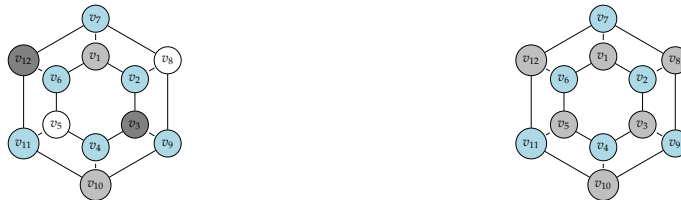
Figure 4.24: Scheduling final exams for twelve classes by coloring a graph of 12 vertices using four colors (left) and coloring the same graph using only two colors (right).
