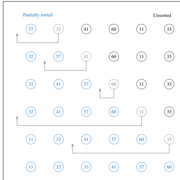
Figure 8.2: A concrete implementation of the insertion sort algorithm.
