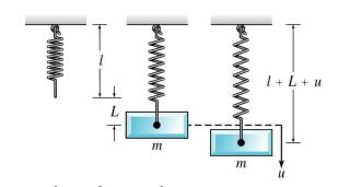
A 4 lb mass stretches a spring 2". The mass is displaced an additional 6" and then released; and is in a medium that exerts a viscous resistance of 6 lb when the mass has a velocity of 3 ft/sec. Formulate the IVP that governs the motion of this mass:
