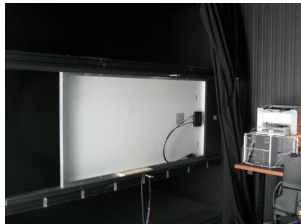
The sun simulator set-up at the PV lab!
