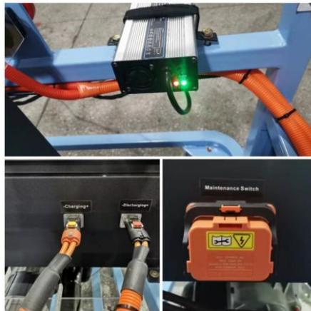
**5. Turn on the 12V power switch:** Turn on the power switch, then charge the battery.
