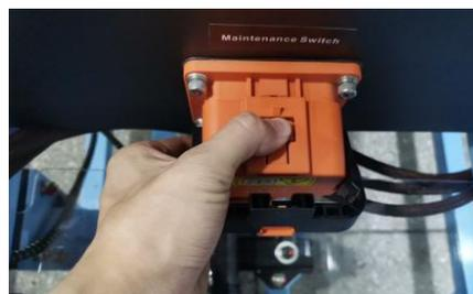
4. While pressing the latch, pull the orange maintenance switch backward to disconnect it.
