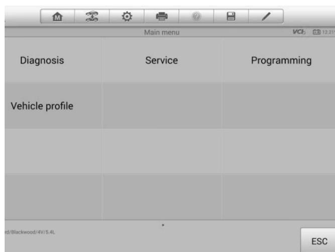
1. Diagnosis – a comprehensive section which includes all available functions: reading, clearing, saving and printing diagnostic information, as well as performing active tests and special functions.
