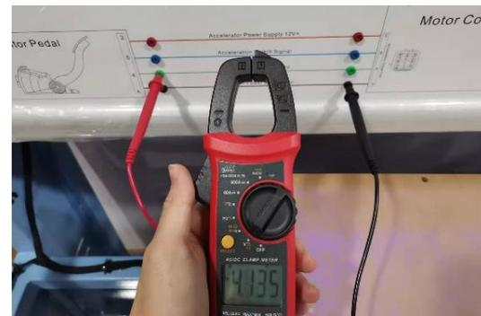
Through the above voltage detection of the line between the accelerator pedal and the motor controller, it can be concluded that the line of the acceleration switch signal is open circuit. Use a wire to connect the two terminals of acceleration switch signal line, press the accelerator pedal and the equipment works normal
