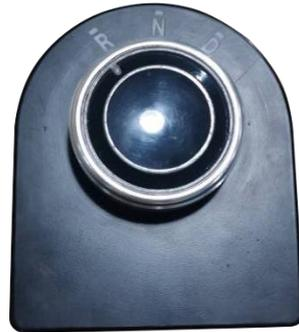
It has three gears R / N / D. According to the driver's intention, the gear position sensor detects the gear position and sends the gear signal to the motor controller. Then the motor controller controls the motor to move forward or reverse or stop.
