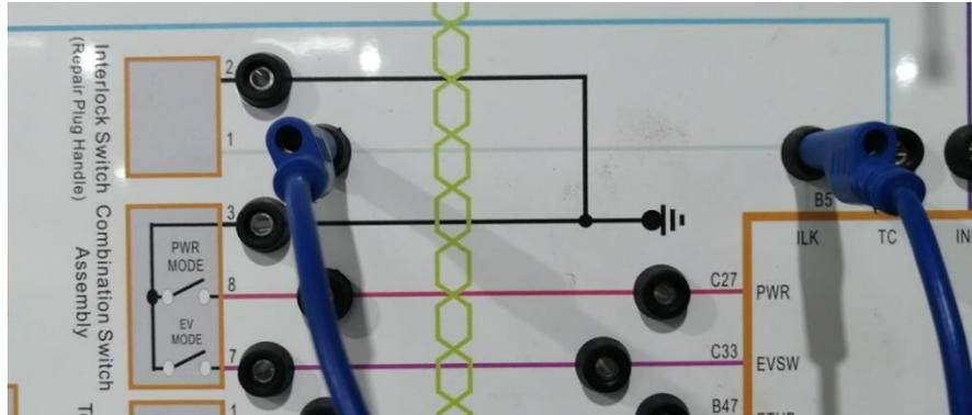
**Fault Conclusion:** The Interlock Switch Line 1 is open circuit.
