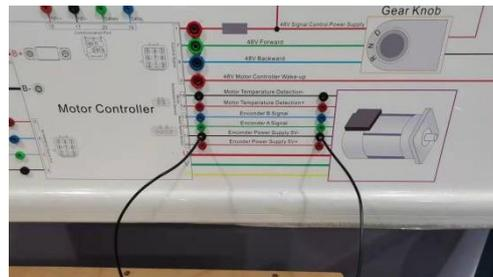
**Conclusion:** Motor Controller Encoder Power Supply 5V- Line is open circuit
