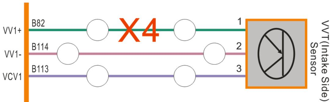
Definition of VVT (Air-intake side) sensor (camshaft position sensor) terminals:
