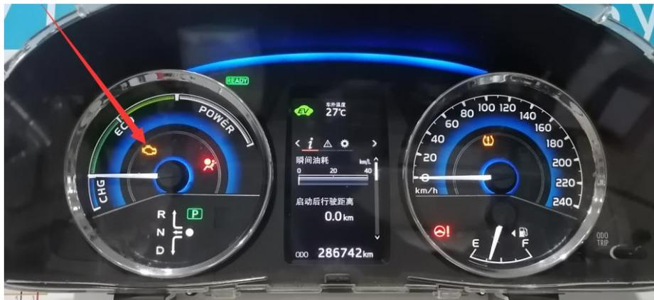
2. Use diagnostic tool to read the fault code P0118, the circuit of engine coolant temperature sensor has high voltage input.
