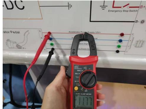
2. Measure the voltage between the accelerator power supply 12V+ (terminal 3) and the accelerator power supply 12V- (terminal 4) on the motor controller side.
