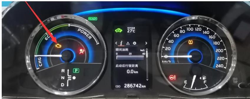
2. Use diagnostic tool to read the fault code P0335, the crankshaft position sensor 'A' circuit.
