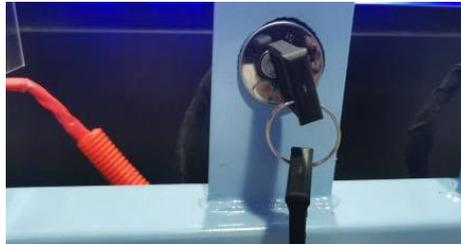
**5. Shift gear:** Select the gear with the gear shift knob. D: forward Direction, R: reverse Direction and N: Neutral (No motion)
