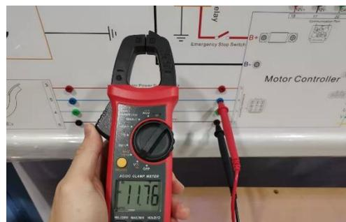
4. Measure the voltage between the acceleration switch signal (terminal 5) and the 12V- ground on the accelerator pedal side.
