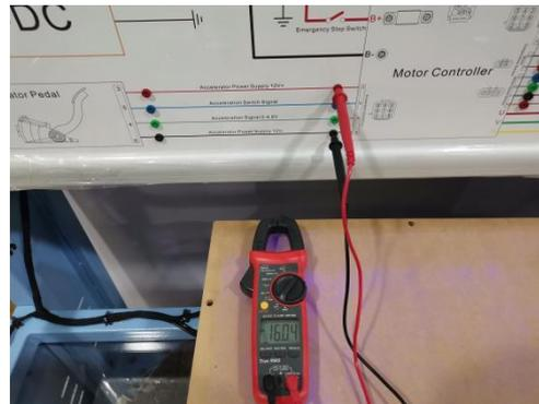
3. Measure the voltage between the accelerator power supply 12V+ (terminal 3) on the accelerator pedal side and the accelerator power supply 12V- (terminal 4) on the motor controller side.
