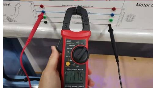
2. Measure the voltage of encoder power supply positive and negative
