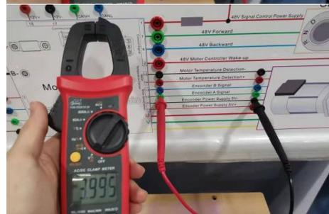
Through the above detection of the line between the accelerator pedal and the motor controller, and the detection of the line between the motor and the motor controller, it can be concluded that the signal line of the encoder B is open circuit. Use a wire to connect the two terminals of encoder B line, and the equipment works normal
