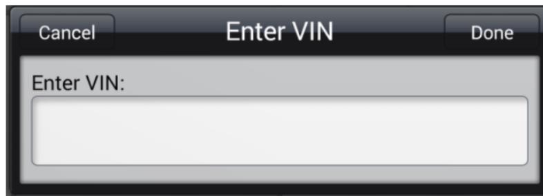
5. Tap **Done**. The vehicle will be identified in a few seconds, and once the matching is successful, the system will guide you to the Vehicle Diagnostics screen directly.
