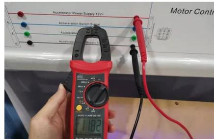
3. Measure the voltage between the acceleration switch signal (terminal 6) and the 12V-ground on the motor controller side.
