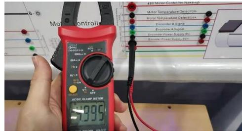
3. Measure the voltage of encoder B signal (EB)
