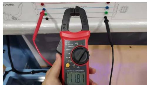
5. Measure the voltage between the acceleration switch signal (terminal 5) and the 12V-ground on the motor controller side.
