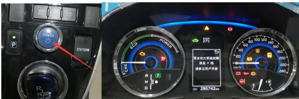
6. Press the brake pedal and press the one-button start switch again. At this time, the power system of the equipment is in the starting state, and the READY indicator is on.
