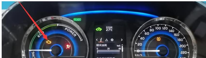
2. Use diagnostic tool to read the fault code P0102, the circuit voltage of air flow meter is low.
