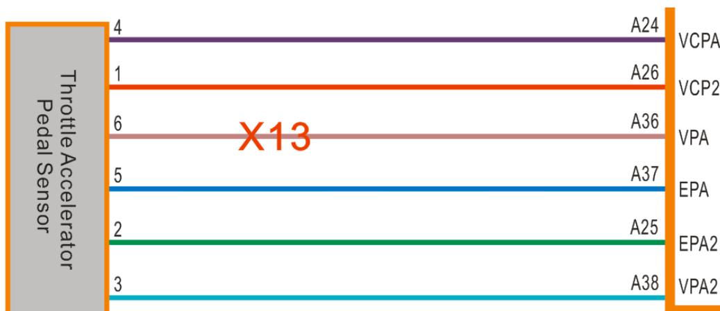
Definition of accelerator pedal position sensor terminals:
