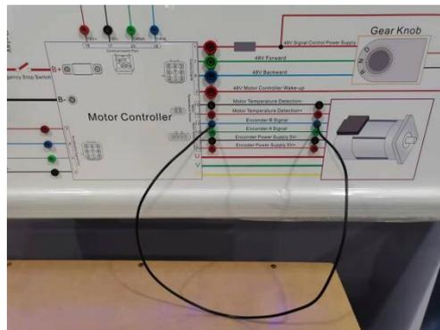
**Conclusion:** Motor Controller Encoder B Signal Line is open circuit
