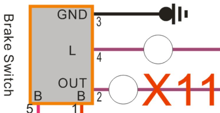
Terminal 2: Brake light switch signal output (the voltage is 11-14V when press the brake pedal, the voltage is 0-1.5V when release the brake pedal)
