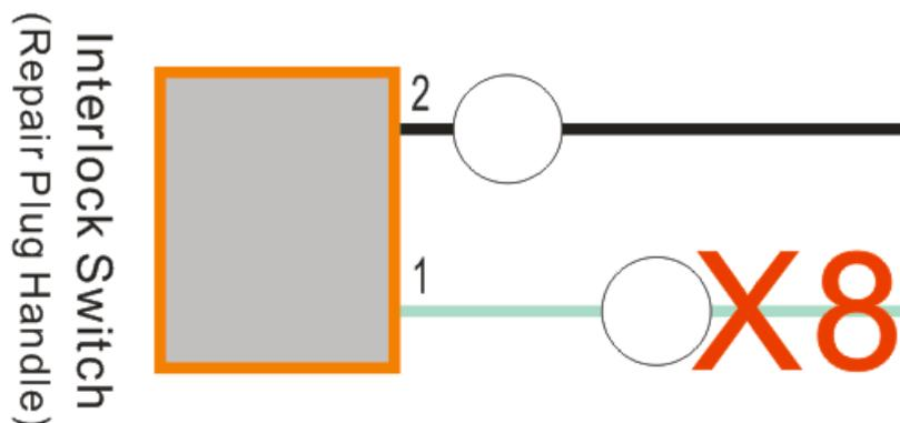
Terminal 1: Interlock switch signal output terminal (When the power switch is in the ON / IG position, and the maintenance plug handle is installed correctly, the standard voltage is 0-1.5V)
