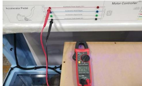
2. Measure the voltage between the accelerator power supply 12V+ (terminal 3) and the accelerator power supply 12V- (terminal 4) on the motor controller side.
