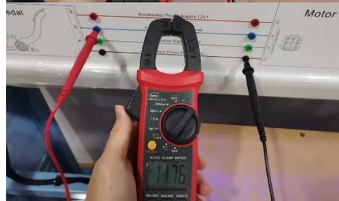
2. Measure the voltage of encoder power supply positive and negative
