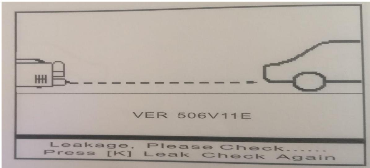
Figure Error! No text of specified style in document..8 leak check fails
