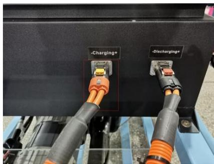
**3. Connect the charger:** Connect the charging bus to the charger, and then connect the charger to the power supply as shown in figure below.
