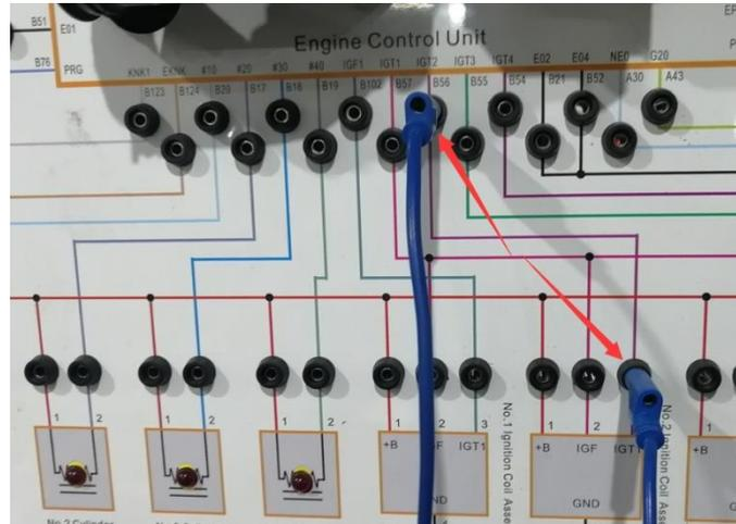
**Fault Conclusion:** The No.2 Ignition Coil Line 3 is open circuit.
