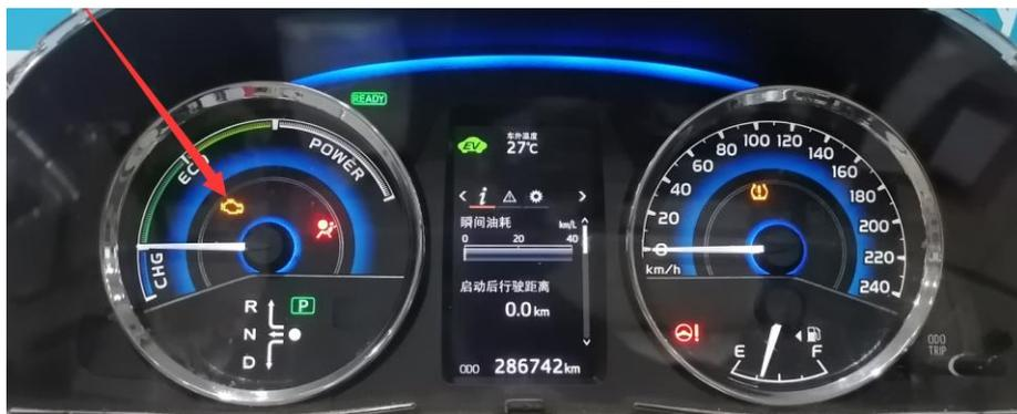
2. Use diagnostic tool to read the fault code P121014/P213800, the throttle / accelerator pedal position sensor has fault.
