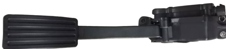
The electronic accelerator pedal converts the driver's driving desire into electronic signal through the electronic structure in the pedal, and transmits it to the motor controller through the signal line. After calculating according to the driver's intention, the motor controller reasonably adjusts the power to achieve the driver's driving purpose.
