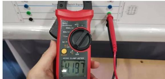
6. Measure the voltage between the acceleration switch signal (terminal 4) and the 12V-ground on the accelerator pedal side.
