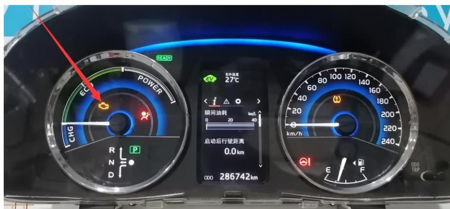
**Fault Conclusion:** The Coolant Temperature Sensor Line 2 is open circuit.
