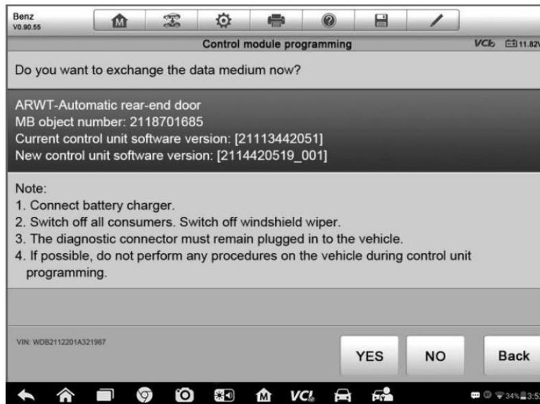
The main section of the reprogramming interface provides you certain hardware version, and current software versions' information, as well as the information of the newest software versions to be programmed to the control units.
