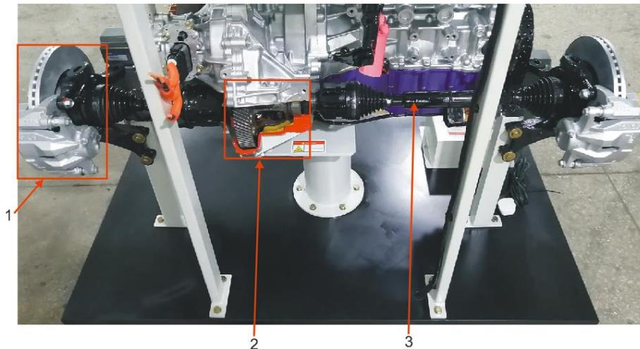
1- Disc brake 2- Main reducer and differential 3- Half shaft
