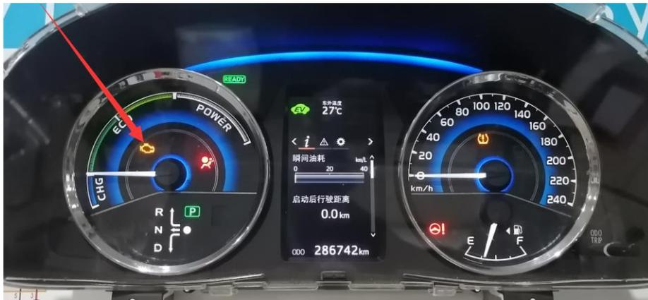
2. Use diagnostic tool to read the fault code P0343, the circuit of camshaft position sensor 'A' has high voltage input.
