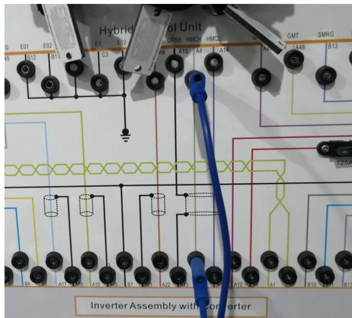
**Fault Conclusion:** The Hybrid Control Unit Line A4 is open circuit.
