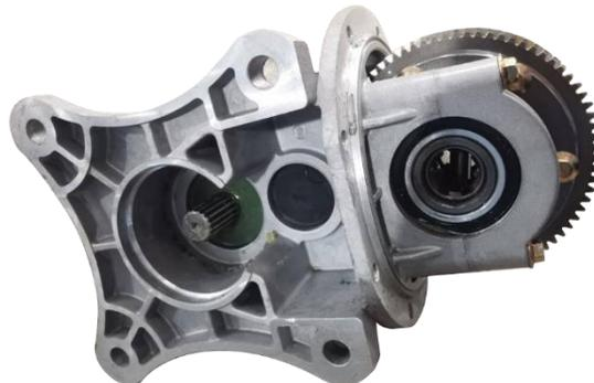
1) The reducer can effectively change the transmission ratio of the whole vehicle, and realize the change of speed and torque. The main function is to reduce the speed and increase the torque of the driving motor. Electric vehicles are generally designed with a two-stage transmission, forward gear and reverse gear sharing structure, and the reverse gear is realized
