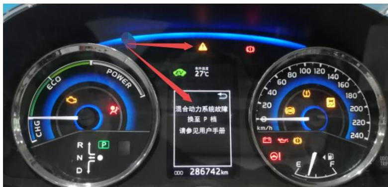
2. Use diagnostic tool to read the fault code P0A0A92, the high voltage system interlock has fault.
