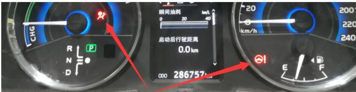
8. The vehicle will put into gear and drive only when “READY” light of the instrument is on. Press the brake pedal and shift the gear to D. The dashboard displays gear D, and it has vehicle speed display, indicating that the vehicle is in forward state.
