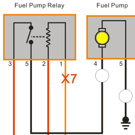
Definition of fuel pump relay terminals:
