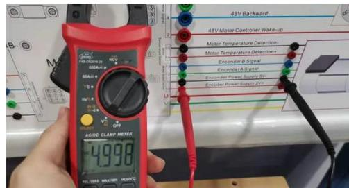
5. Measure the voltage across the encoder power supply 5V- terminals, and the voltage across the encoder power supply 5V+ terminals.
