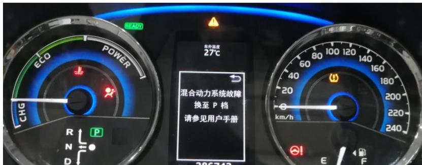
2. Use diagnostic tool to read the fault code P312387, Communication error / lost communication from the drive motor control module to the hybrid / EV transmission system control module.
