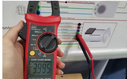
Through the above detection of the line between the accelerator pedal and the motor controller, and the detection of the line between the motor and the motor controller, it can be concluded that the line of the encoder power supply 5V+ is open circuit. Use a wire to connect the two terminals of encoder power supply 5V+ line, and the equipment works normal
