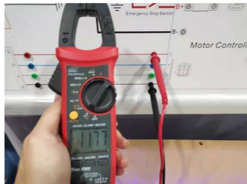
3. Measure the voltage between the acceleration switch signal (terminal 6) and the 12V- ground on the motor controller side.
