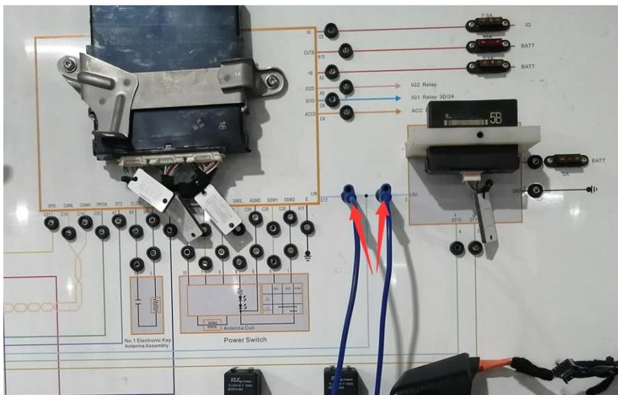
According to the above diagnosis, it can be determined that the line between the identification code box terminal 2 (LIN1) and smart key certified ECU terminal C17 (LIN) is open circuit.
