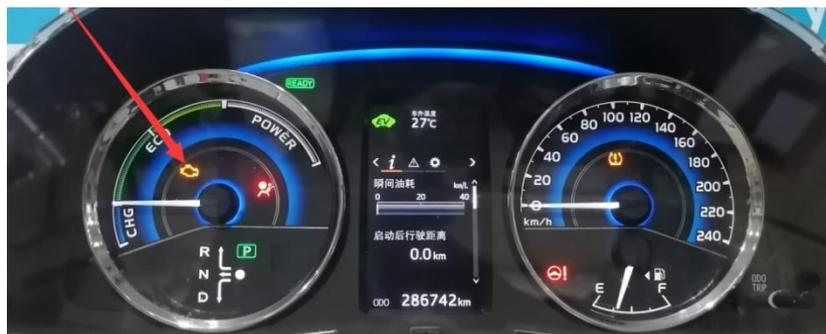
3. Use diagnostic tool to read the fault code P0352, the ignition coil 'B' primary / secondary circuit.
