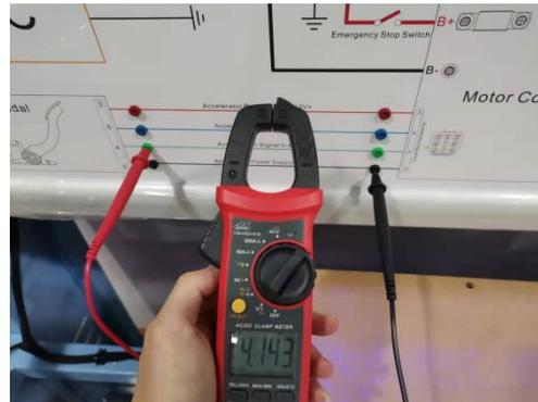
Through the above voltage detection of the line between the accelerator pedal and the motor controller, it can be concluded that the line of the accelerator pedal signal 0-4.8V is open circuit. Use a wire to connect the two terminals of accelerator pedal signal 0-4.8V line, press the accelerator pedal and the equipment works normal
