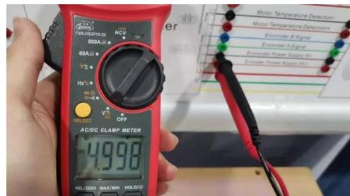
3. Measure the voltage of encoder power supply positive and negative: From the motor side, measure the voltage between the encoder power supply 5V+ and the encoder power supply 5V-.
