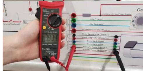
Through the above detection of the line between the accelerator pedal and the motor controller, and the detection of the line between the motor and the motor controller, it can be concluded that the signal line of the encoder A is open circuit. Use a wire to connect the two terminals of encoder A line, and the equipment works normal
