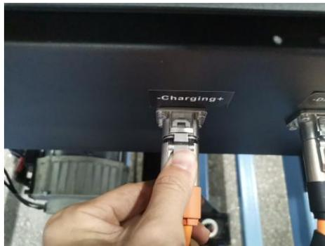
3. Release the latch after it exits the charging socket.
