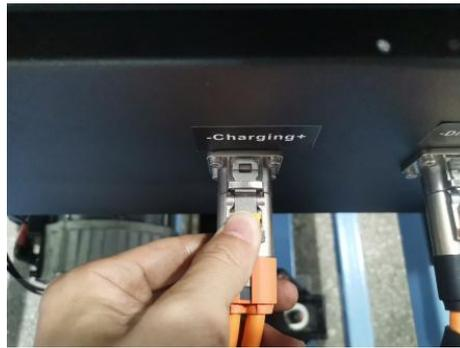
2. Pull out part of the connector from the charging socket.
