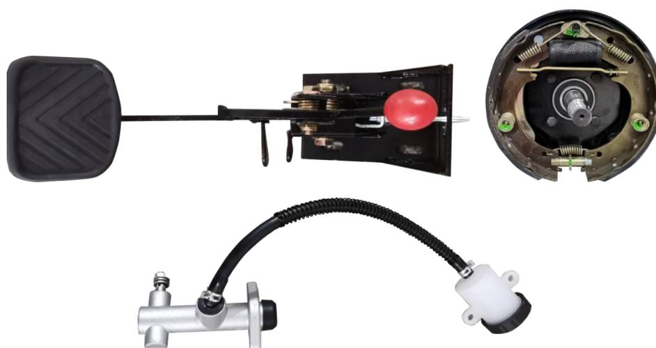
Drum brakes and hydraulic brake system are adopted. When braking, the brake pedal pushes the hydraulic oil in the brake hose to form oil pressure to open the drum brake pads. At this
