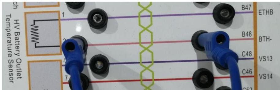
**Fault Conclusion:** The HV Battery Outlet Temperature Sensor Line 2 is open circuit.
