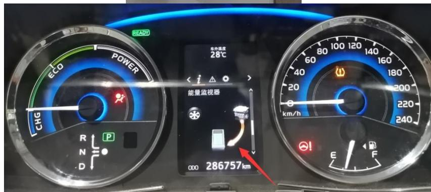
10. Press the brake pedal and shift the gear to R. The dashboard displays gear R, and it has vehicle speed display, indicating that the vehicle is in reverse state.
