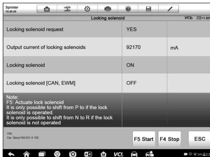
The functional buttons at the lower right corner of the Active Test screen manipulate the test signals. The operational instructions are displayed on the main section of the test screen. Simply follow the on-screen instructions and make appropriate selections to complete the tests. Each time when an operation is successfully executed, message such as “Command Finished”, “Activation Successful”, or something similar displays.
