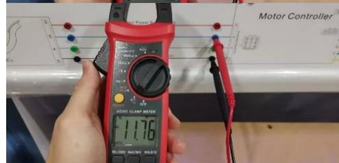
2. Measure the voltage of encoder power supply positive and negative: From the motor controller side, measure the voltage between the encoder power supply 5V+ and the encoder power supply 5V-
