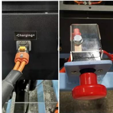
**2. Connect the charging bus:** Connect the charging bus to the battery pack charging interface as shown in figure below.
