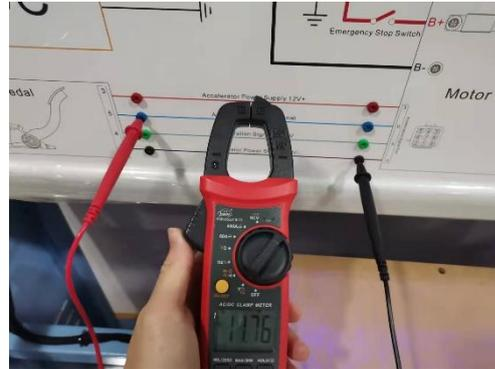
5. Measure the voltage between the acceleration signal (terminal 5) and the 12V- ground on the motor controller side.
