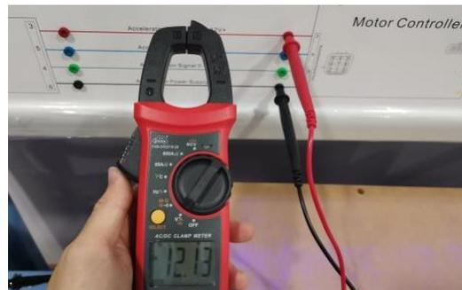
3. The voltage between the accelerator power supply 12V+ (terminal 3) on the accelerator pedal side and the accelerator power supply 12V- (terminal 4) on the motor controller side.
