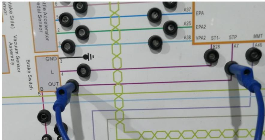
**Fault Conclusion:** The Brake Switch Line 2 is open circuit.
