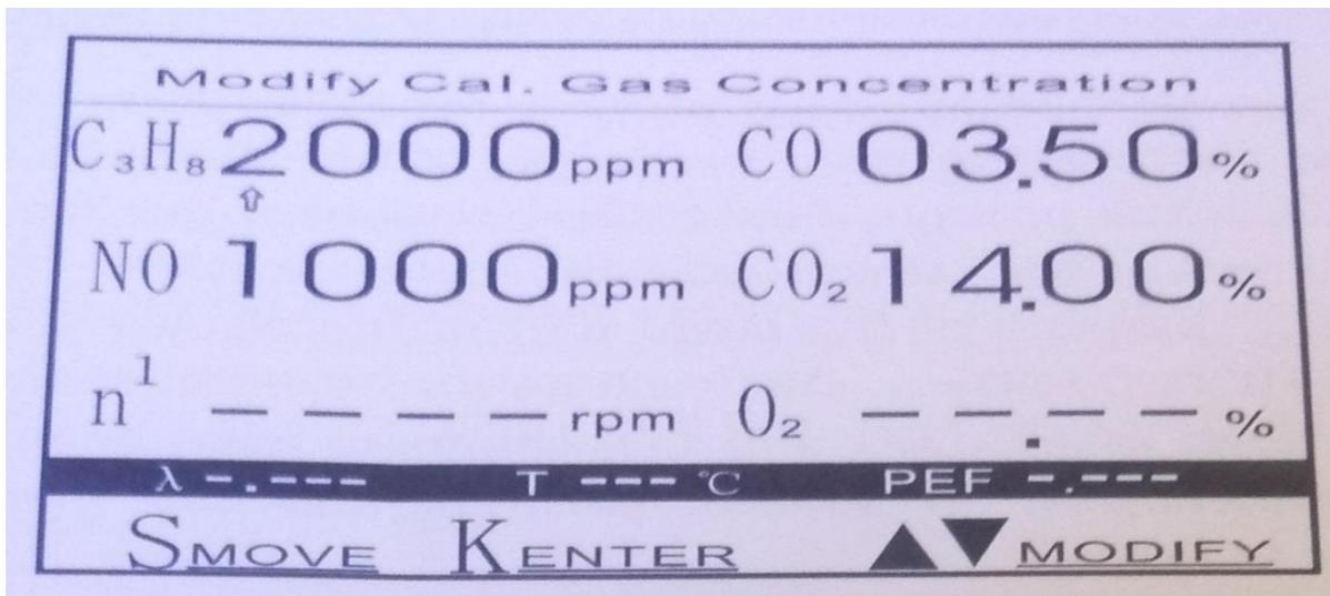
Figure Error! No text of specified style in document..14 Modify Concentration of calibration gas
