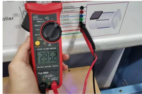
4. Measure the voltage between the encoder power supply 5V+ terminals from the motor controller side, and the encoder power supply 5V- terminals from the motor side.
