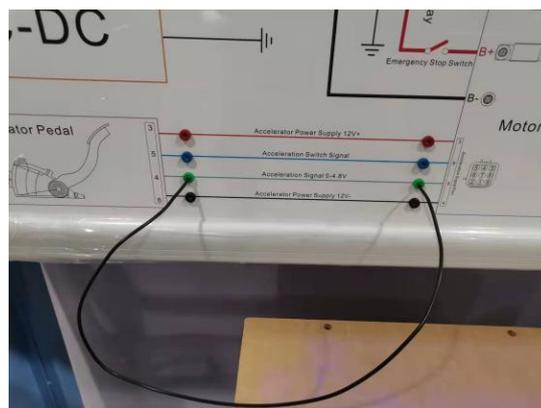
**Conclusion:** Accelerator Pedal Signal Line 0-4.8V is open circuit
