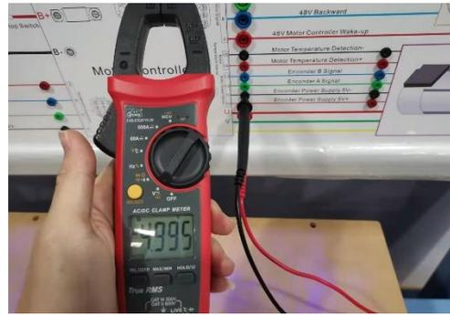
3. Measure the voltage of encoder B signal (EB)
