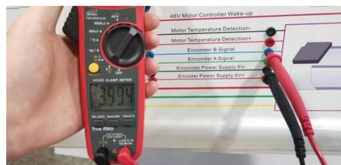
7. Measure the voltage of encoder A signal (EA): From the motor side, measure the voltage between encoder A signal and encoder power supply 5V-.
