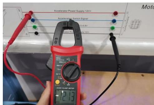
4. The voltage between the accelerator power supply 12V+ (terminal 3) on the motor controller side and the accelerator power supply 12V- (terminal 6) on the accelerator pedal side.
