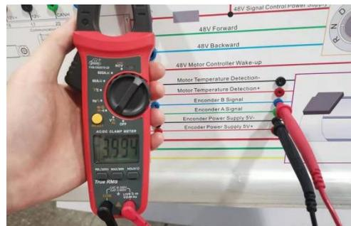
4. Measure the voltage of encoder A signal (EA)
