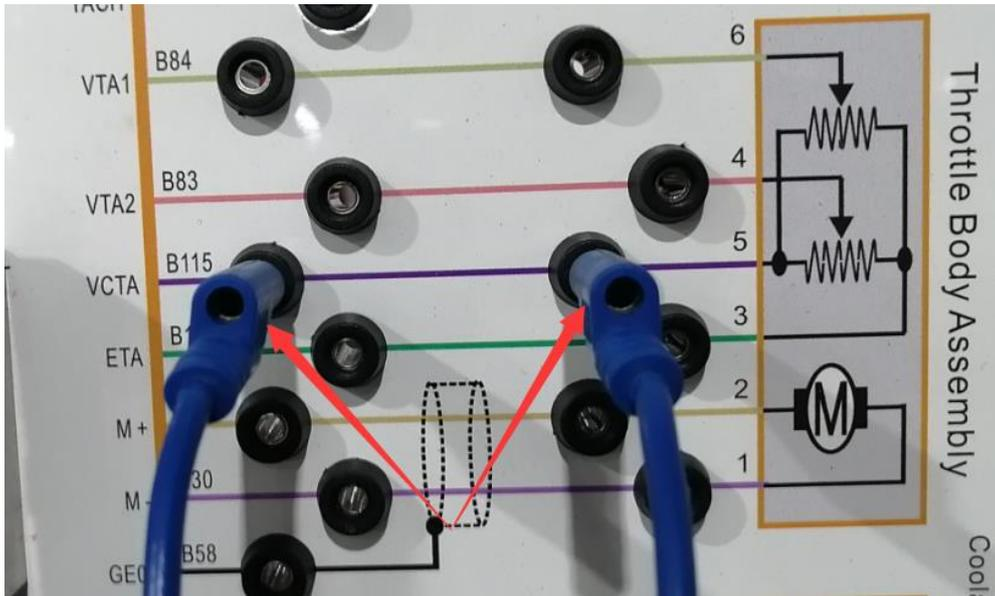
**Fault Conclusion:** The Throttle Body Assembly Line 5 is open circuit.
