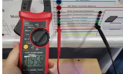
3. Measure the voltage of encoder B signal EB
