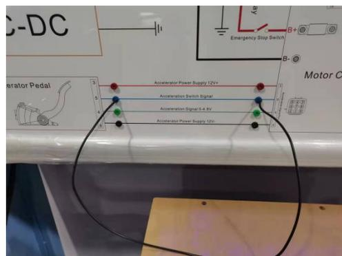
**Conclusion** : Acceleration Switch Signal Line is open circuit
