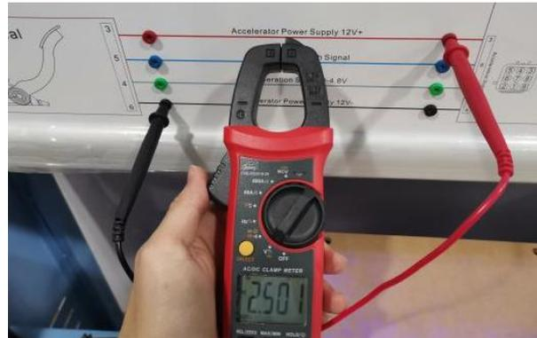
Through the above voltage detection of the line between the accelerator pedal and the motor controller, it can be concluded that the line of the accelerator power supply 12V- is open circuit. Use a wire to connect the two terminals of accelerator power supply 12V- line, press the accelerator pedal and the equipment works normal
