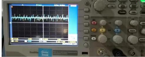
2. Measure the waveforms of CANH and CANL at the motor controller terminals by oscilloscope
