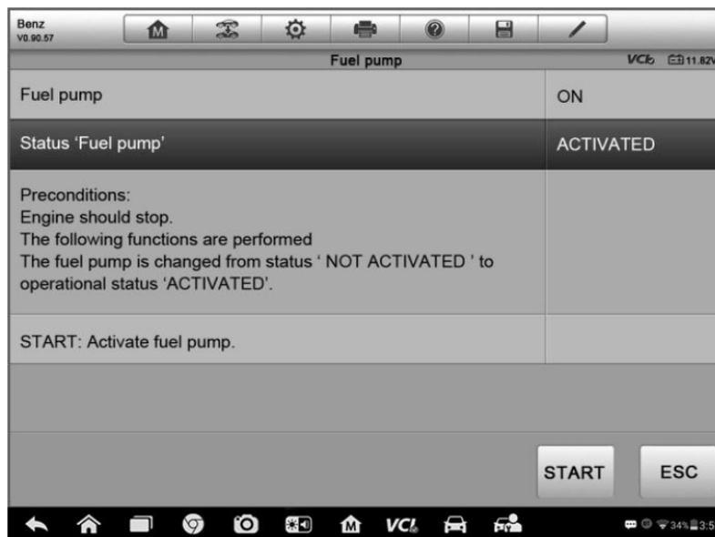
Read the information carefully and check the vehicle condition accordingly, when you are sure that the vehicle is ready to perform the adaptation, simply follow the instruction provided to make appropriate selections. When the operation is done, an execution status message such as Completed, Finished or Successful, displays.
