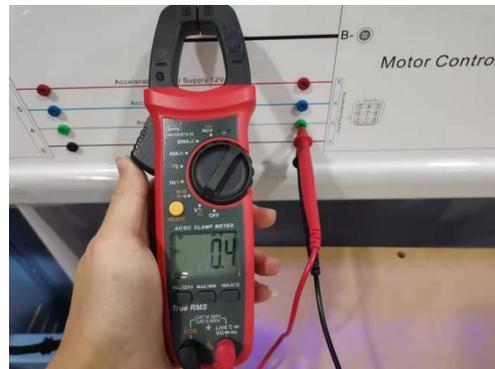
6. Measure the voltage between the acceleration signal (terminal 4) and the 12V- ground on the accelerator pedal side.
