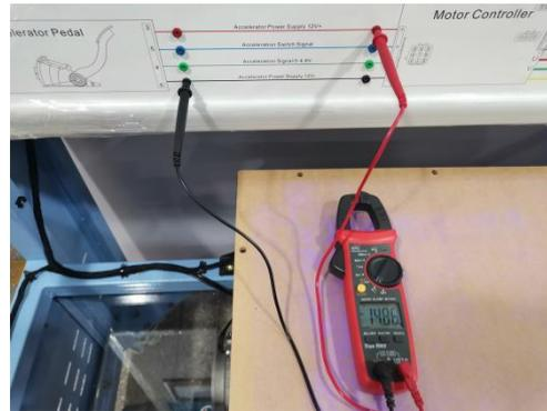
Through the above voltage detection of the line between the accelerator pedal and the motor controller, it can be concluded that the line of the accelerator power supply 12V+ is open circuit. Use a wire to connect the two terminals of accelerator power supply 12V+ line, press the accelerator pedal and the equipment works normal
