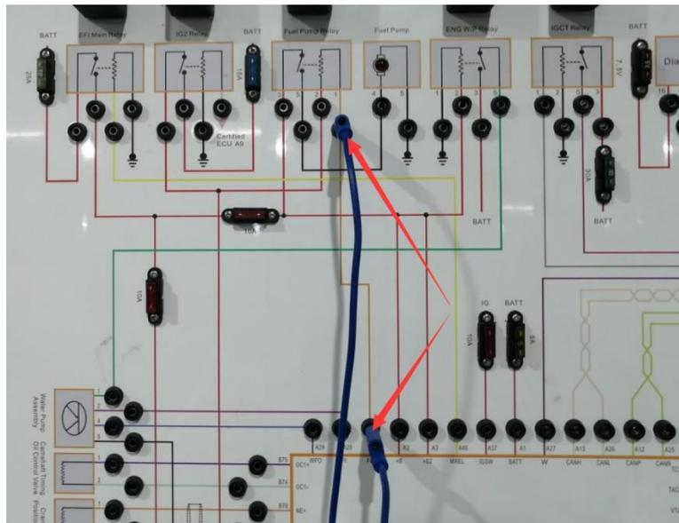
**Fault Conclusion:** The Fuel Pump Relay Control Line is open circuit.
