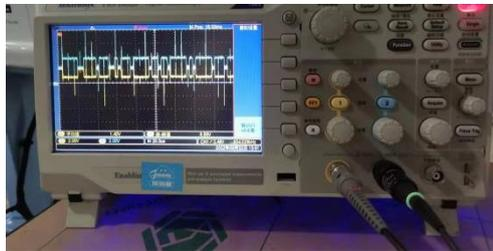
Through the waveforms measurement by oscilloscope at the dashboard and motor controller terminals, it can be seen that there is no waveform of CANL at dashboard terminals, it can be judged that the CANL line is open circuit. Use a wire to connect the terminals of motor control CANL and dashboard CANL, the dashboard works normal. So the line is open circuit.
