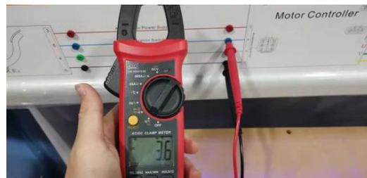
4. Measure the voltage between the acceleration switch signal (terminal 5) and the 12V-ground on the accelerator pedal side.
