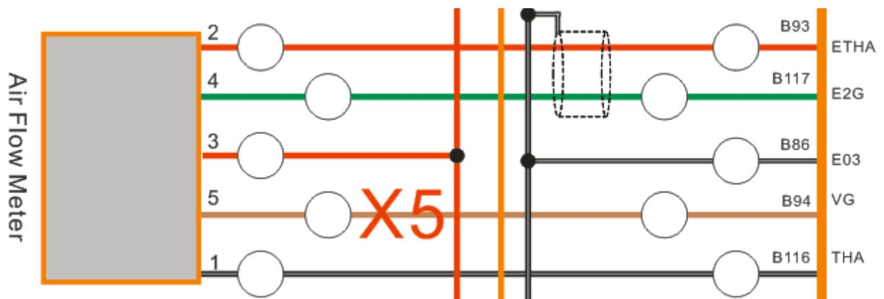
2. Open the ignition switch, connect the decoder and read failure code P0102.
