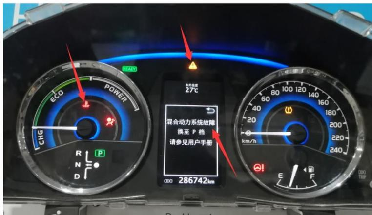
2. There is no response when press the accelerator pedal.
