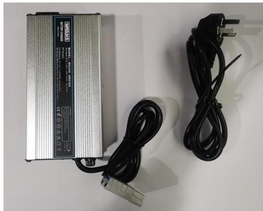
When charging, the BMS receives the charging signal from the charging port, and the BMS detects the battery voltage, current, temperature and balance state, then analyzes and calculates the battery power according to these battery parameters. The 220V high-voltage AC is converted into high-voltage DC in the charger to charge the power battery. Please turn on the power switch to wake up the BMS, then it starts charging.
