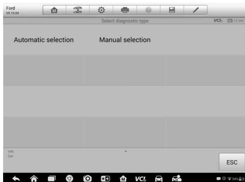
Select **Automatic Selection** and the system will proceed to acquire VIN information automatically or allow users to input the VIN manually.
