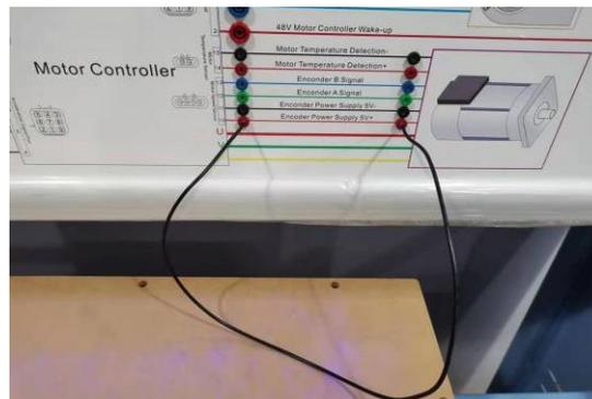
**Conclusion:** Motor Controller Encoder Power Supply 5V+ Line is open circuit
