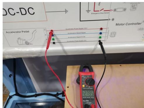
4. Measure the voltage between the accelerator power supply 12V+ (terminal 3) on the motor controller side and the accelerator power supply 12V- (terminal 6) on the accelerator pedal side.
