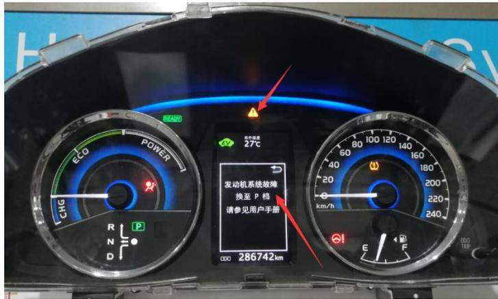
3. Use diagnostic tool to read the fault code P0121/P0122/P0222/P2135, throttle pedal / position sensor has fault
