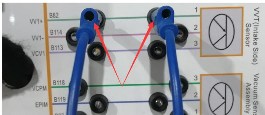
**Fault Conclusion:** The VVT (Air-intake Side) Sensor Line 1 is open circuit.
