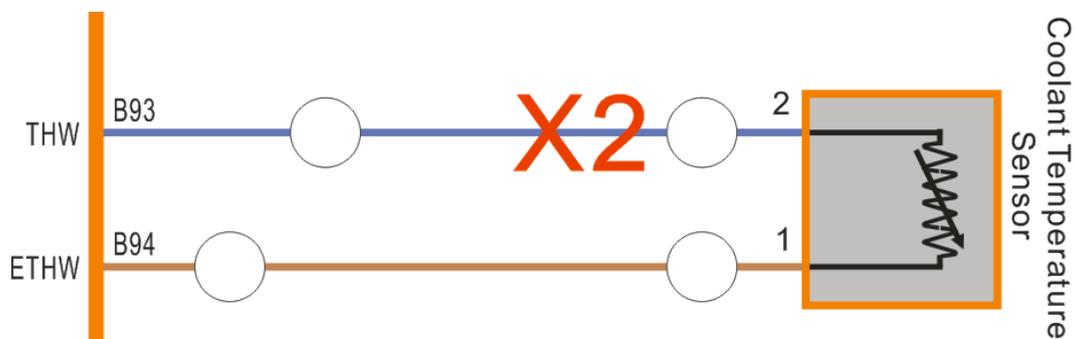
Definition of coolant temperature sensor terminals:
