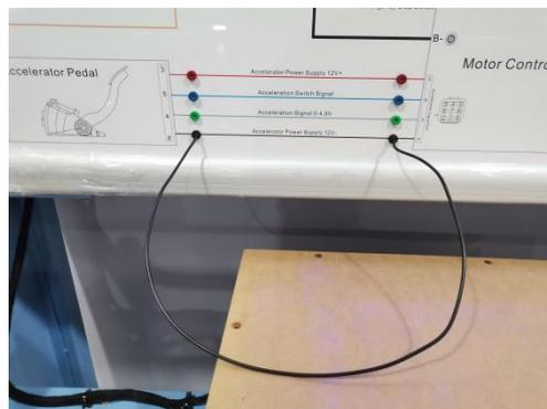
**Conclusion :** Accelerator Power Supply 12V- Line is open circuit
