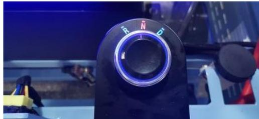
**6. Accelerate:** After selecting D on the gear shift knob, Press the accelerator pedal, the driving motor can run, and the speed can be checked through the dashboard.
