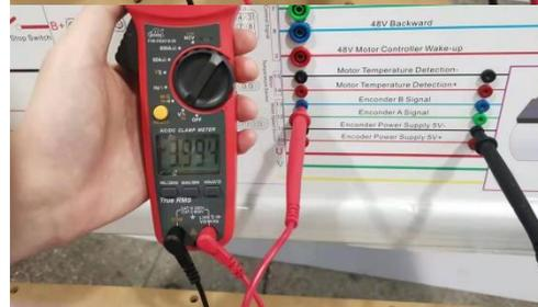
4. Measure the voltage of encoder A signal (EA)
