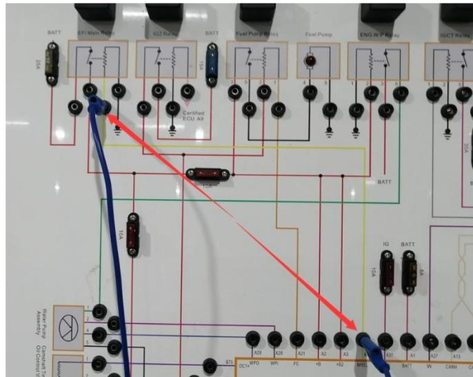
**Fault Conclusion:** The EFI Main Relay Control Line is open circuit.
