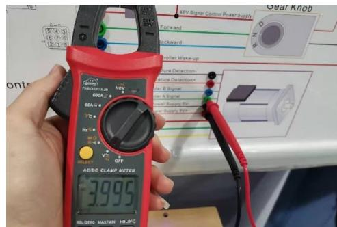
Through the above detection of the line between the accelerator pedal and the motor controller, and the detection of the line between the motor and the motor controller, it can be concluded that the line of the encoder power supply 5V- is open circuit. Use a wire to connect the two terminals of encoder power supply 5V- line, and the equipment works normal
