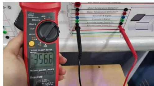
6. Measure the voltage of encoder B signal (EB): From the motor side, measure the voltage between encoder B signal and encoder power supply 5V-
