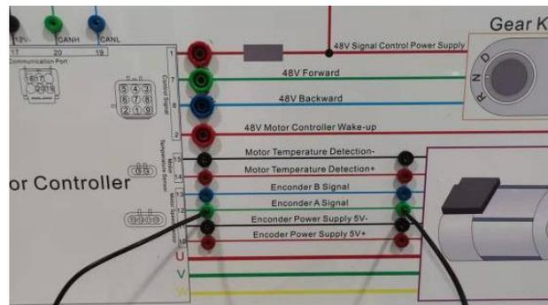
**Conclusion:** Motor Controller Encoder A Signal Line is open circuit
