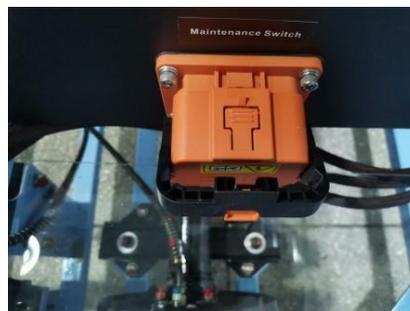
3. Press down the latch on the top of the orange maintenance switch to release it.
