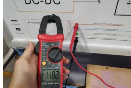
2. Measure the voltage between the accelerator power supply 12V+ (terminal 3) and the accelerator power supply 12V- (terminal 4) on the motor controller side.
