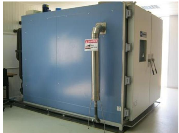
The environmental chamber at the PV technology laboratory
